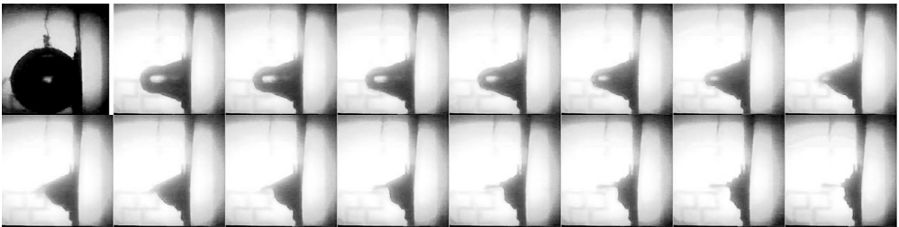
FIGURE 9. Bubble shape before collapse, 2FI boundary, \gamma=0.71 , D=1.5 m, frame interval = 0.2 ms, image width = 500 mm; first image is the bubble at maximum.
